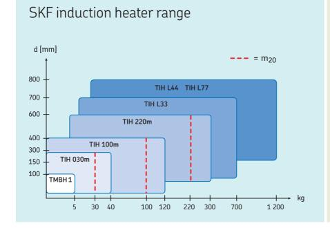
The comprehensive range of SKF induction heaters is suitable for most bearing heating applications. The chart gives general information on choosing an induction heater for bearing heating applications <sup>3</sup>).
